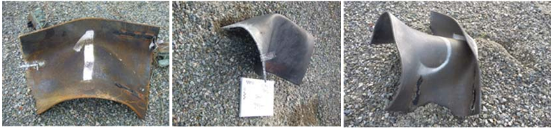
Figure 6 Deformation of the doors in the 1/5th scale test for test 1 (no earth cover), and test 2 and 5 (with an earth cover).
