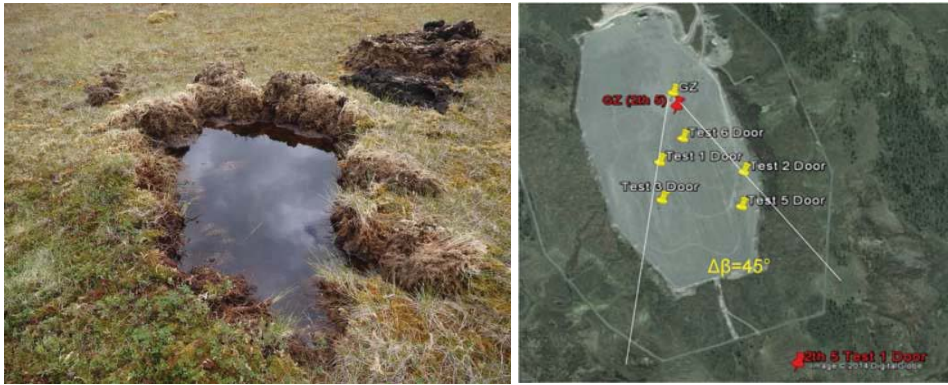
Figure 8 Impact crater in swamp in the 2/5 th scale test (left). Door impact distances in 1/5 th and 2/5 th scaled test (right).
