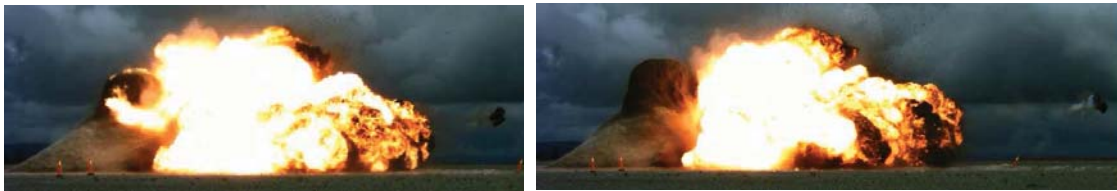
Figure 7 High speed video recordings of the door launch in the 2/5th scale test.
