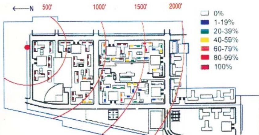
Fig. 15. Patio door glass breakage at the Khobar tower compound [18].
