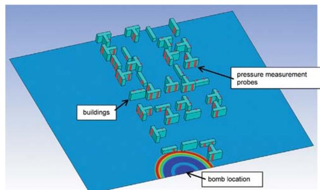
Fig. 17. Simulation setup showing the bomb (bottom), buildings and pressure measurement probe locations (red). (For interpretation of the references to color in this figure legend, the reader is referred to the web version of the article.)
