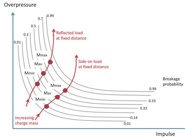
Fig. 13. Schematic  $P-i$  curves for glazing together with load curves for a fixed distance and varying charge mass. Probabilities have been selected for the two cases outlined in Fig. 10, and based on Fig. 12.
