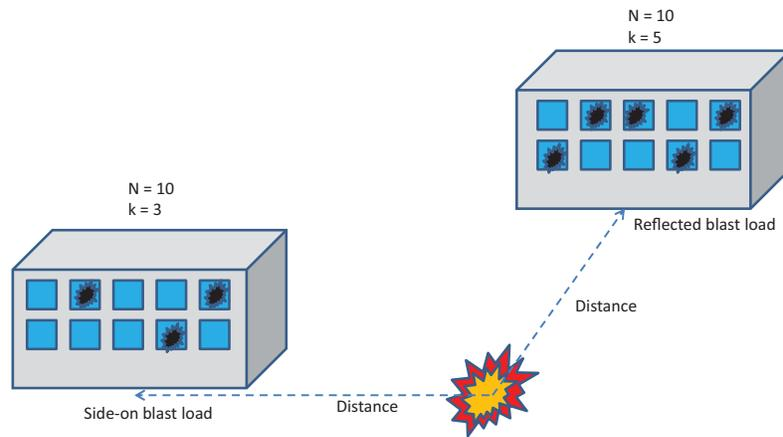
Fig. 10. Two examples of window breakage.
