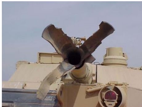
Artillery projectile gun launch and barrel damage as a result of prematures
