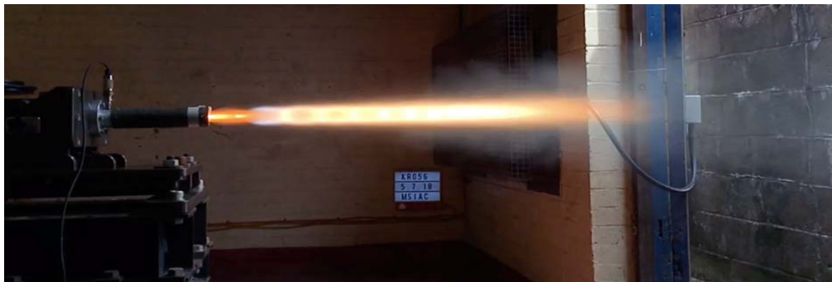
A RAM-mixed Falcon K round being fired during the MSIAC visit; picture courtesy of The Falcon Project ©
