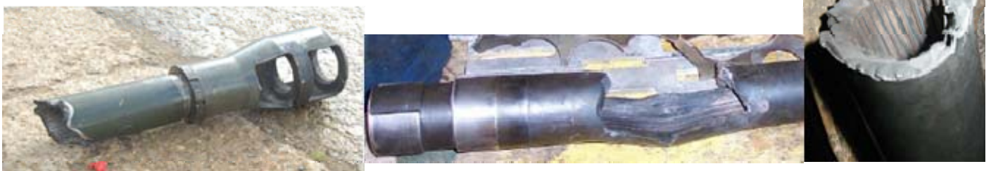
Resulting Gun Barrels from Catastrophic In-Bore Prematures
