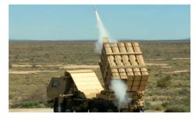
called Integrated Fire Protection Capability. The MML launcher can rotate 360 degrees and elevate from 0-90 degrees in order to identify and knock out approaching fire from any direction or angle.
