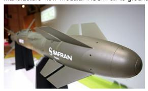
France and other countries, give precision guidance to standard bombs and come in several versions, depending on the type of guidance: inertial GPS, inertial/GPS + infrared imaging, and inertial/GPS + laser, DGA said in a statement Thursday.
