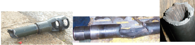
Resulting Gun Barrels from Catastrophic In-Bore Prematures
