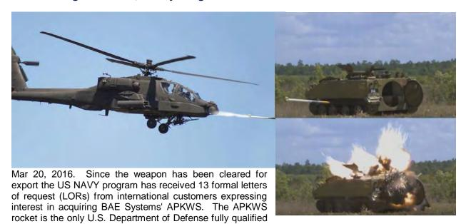
guided 2.75-inch rocket. It uses semi-active laser guidance technology to strike both soft and lightly armored targets in confined areas, providing greater accuracy and mission effectiveness.
