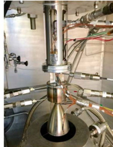
The 200N thruster in the vacuum test stand.
