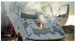
The demonstration marked the first field testing of an integrated 30-kilowatt, single-mode fiber laser weapon system prototype. Through a technique called spectral beam combining, multiple fiber laser modules form a single, powerful, high-quality beam that provides greater efficiency and lethality than multiple individual 10-kilowatt lasers used in other systems.
