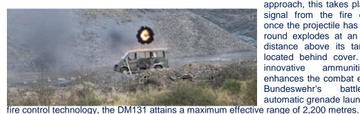
approach, this takes place via an infrared signal from the fire control/aiming unit once the projectile has left the barrel. The round explodes at an exactly calculated distance above its target, even if it is located behind cover. As a result, this innovative ammunition substantially enhances the combat effectiveness of the Bundeswehr's battle-proven automatic grenade launcher. With the right
