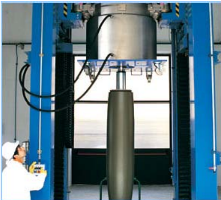
BLU-117 General Purpose Bomb Being Filled with Cast-cured Explosive PBXN-109
