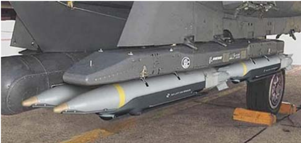
Rack of Four Small Diameter Bombs (SDB I) on a F-15 Aircraft
