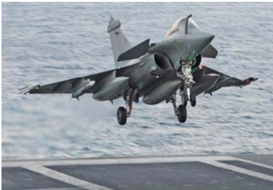
A French Navy Rafale M lands onboard the carrier Charles de Gaulle during Meteor trials
