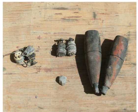
Shell bodies and separated M783 fuzes from M768 cartridges were recovered from SPC Alan Ng's vehicle after the Sept. 12, 2009, MRAP fire.
