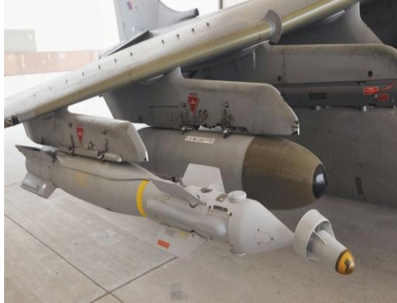
Paveway IV Loaded on a RAF Harrier GR.Mk 9A at Kandahar in
