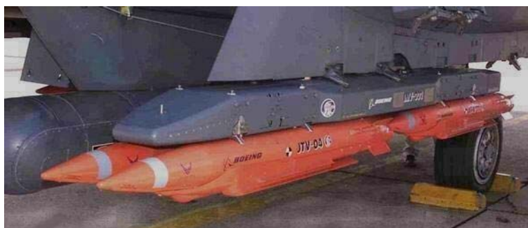
Carriage to fit 4 SDB Units in the Bay of an F-22 Aircraft
